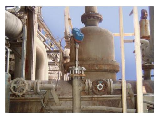
Buffer tanks are usually located between process installations to help reduce the impact of flow changes between interconnected process installations. Too low level of buffer tank will lead to reduced output, and too high level will lead to liquid material carry-over. In applications characterized by alternating inertia and turbulence, stable level output is highly desirable.
